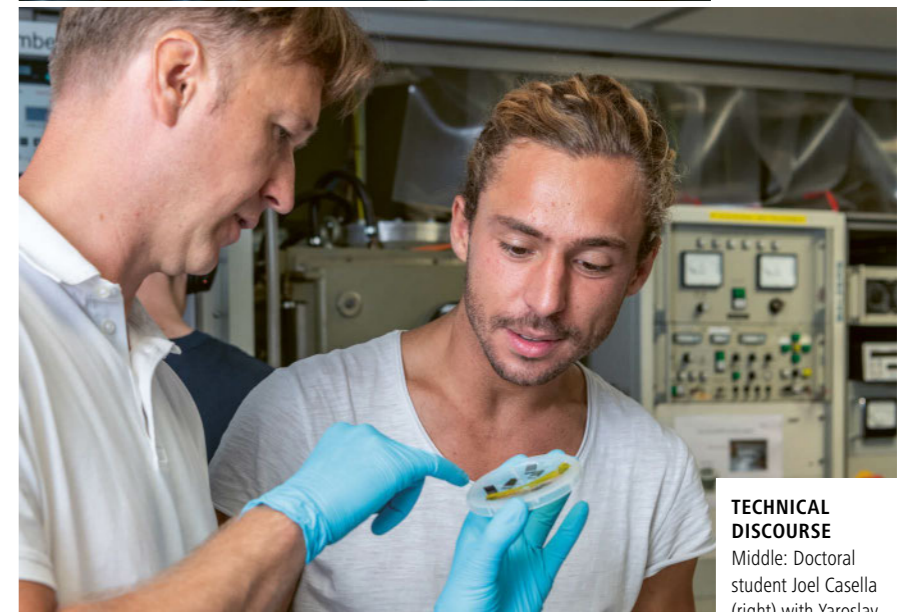
FILIGREE Two-layer cathodes for thin-film solid-state batteries are deposited on the substrate.
