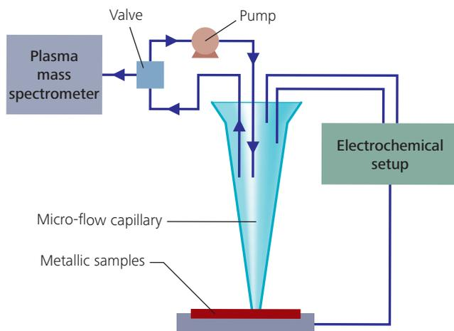
Principle of the newly developed analytical setup: a thin capillary is placed on the sample, and filled with a corrosive medium (e.g. a saline solution). At defined time intervals, a small amount of the solution is taken from the capillary and sent to a plasma mass spectrometer to determine the different dissolution rates of the individual elements.
