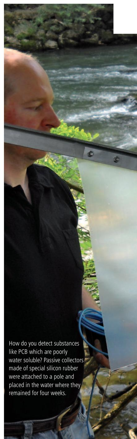
How do you detect substances like PCB which are poorly water soluble? Passive collectors made of special silicon rubber were attached to a pole and placed in the water where they remained for four weeks.
